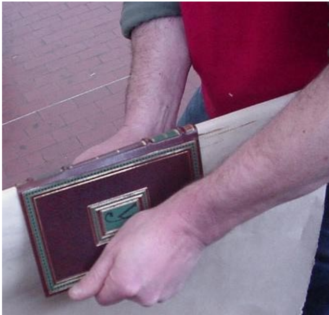
The expert hands of Luigi Biffi putting the convexity in the spine of volume 1 over a bar of hot iron. The leather used for VIE books is from Mountain Rams. Photo by Brian Gharst.
